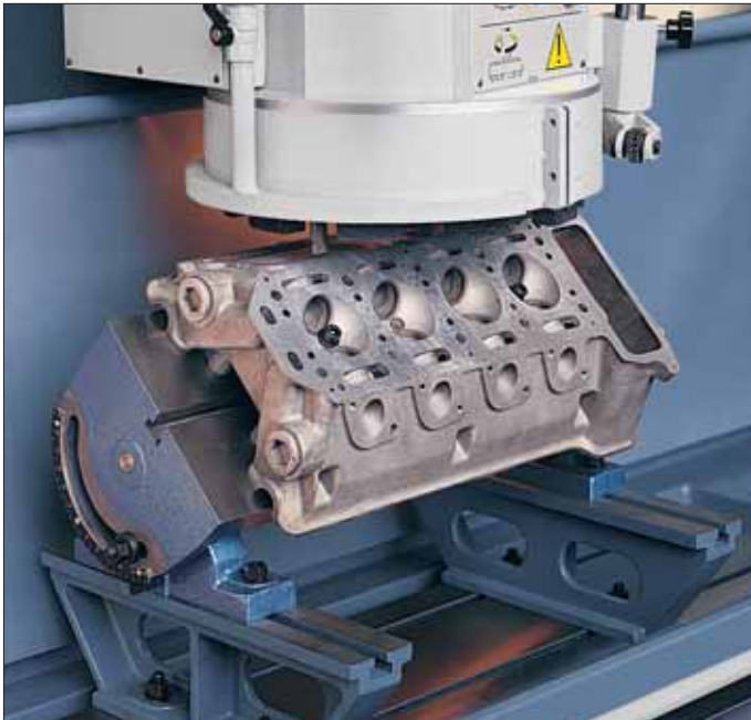
Fig. 1 Reconditioning of manifold mating surfaces with insert type milling tool. The head is clamped on the universal square.
