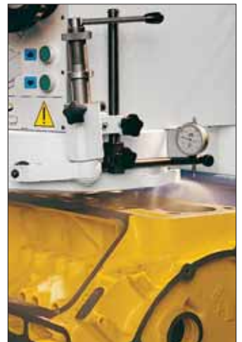
Grinding a cylinder block with segmental wheel.
