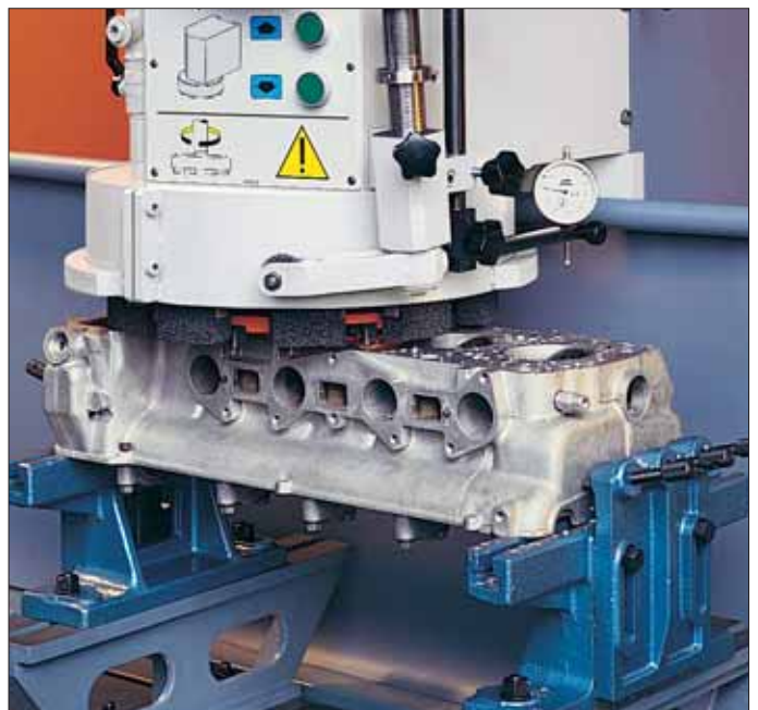
Fig. 2 Milling a cylinder head using insert type milling cutter.
